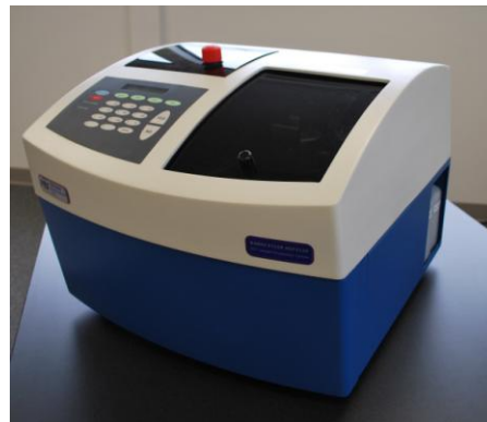
Figure 1. Barocycler NEP 2320. This instrument generates cycles of hydrostatic pressure up to 35,000 psi (240 MPa) and accommodates one PULSE Tube (1.5 mL) or up to 12 smaller MicroTubes (50-150 \mu L) at a time. A larger instrument, Barocycler NEP 3229 is available, which accommodates 3 or 48 samples, respectively.
