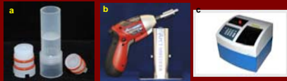
Figure 1. The PCT Shredder Tube™, Shredder Stand and tool for grinding tissue samples. (a) Tissue samples are loaded into the bottom of the tube (top in picture) and sealed in with a ram (right of tube). The extraction liquid is then added to the tube (bottom in picture) closed with the lid (left of tube). (b) The tube is seated in the PCT Shredder stand and ground using the grinding tool before being placed into (c) the NEP2320 Barocycler for pressure cycling
