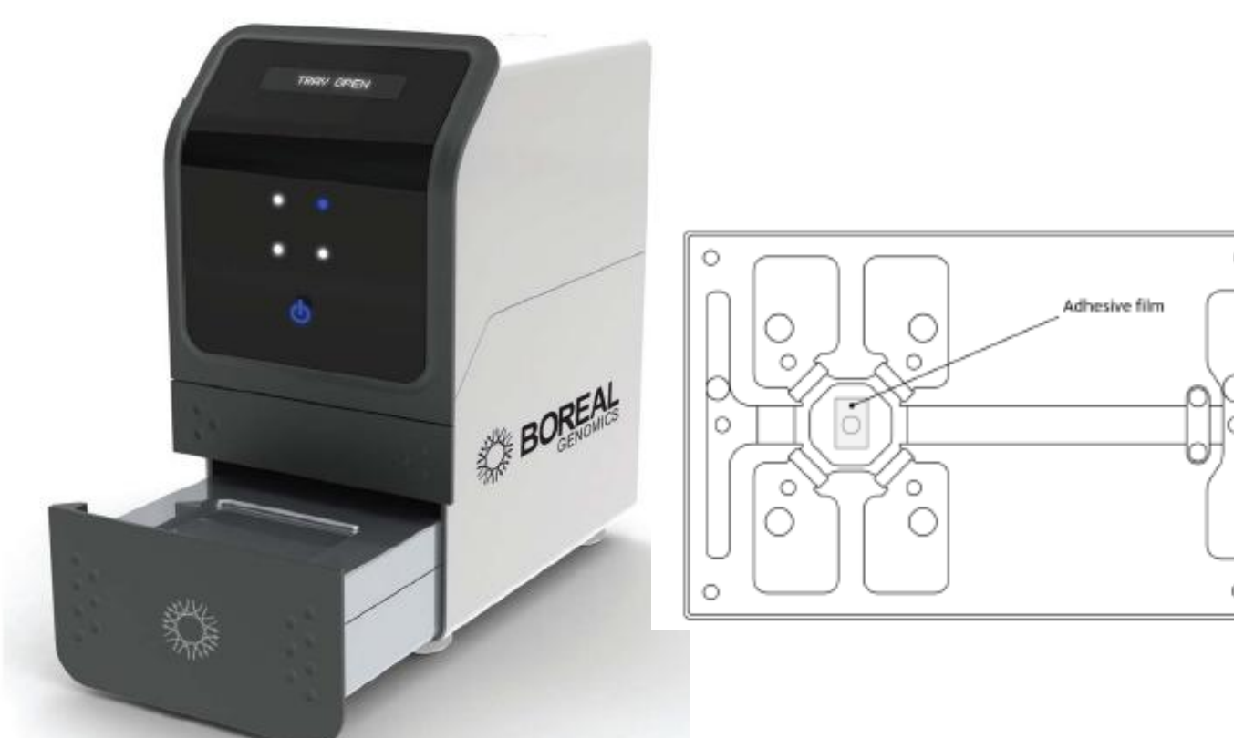
Figure 5. SCODA Instrument and Sample Cartridge. The custom cartridges consist of a 5 mL injection chamber (60 mm long, 7 mm deep and 12 mm wide), a concentration gel casting region, and a 15 mL electrophoretic buffer reservoir for each of the four electrodes that generate the rotating fields. Figure used with permission from Boreal Genomics.
