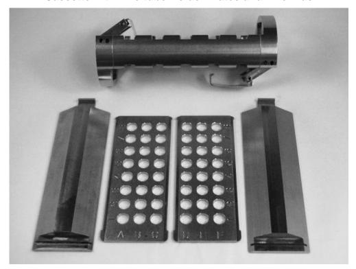
Cassette with Tube Holder Plate and Three BaroFlex Strips in Place
